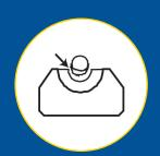
100% thermal contact between the pipe freezer head and the pipe to be frozen is essential to a successful freeze. If the freeze-head does not have proper contact with the pipe, the freeze may not form.
